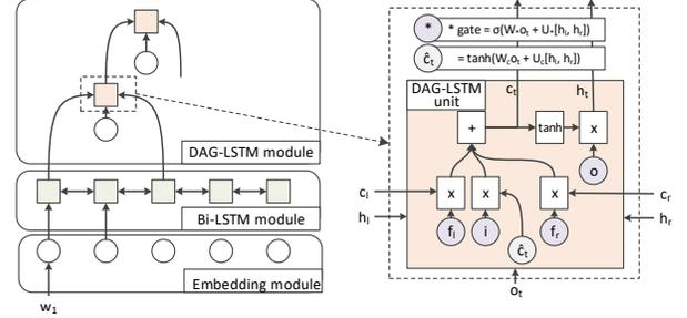
Figure 6: Our iterative relation extraction model. Overview on left and details of DAG-LSTM unit on right.
